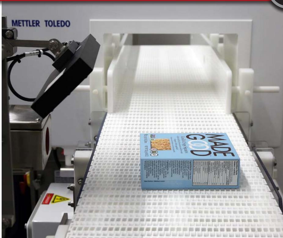
A box of Made Good granola bars, produced by Shawpak System's long-time client Riverside Natural Foods, gets a thorough once-over from the METTLER-TOLEDO CI-Vision brand machine vision system to verify all the critical product and coding information printed on the package.
